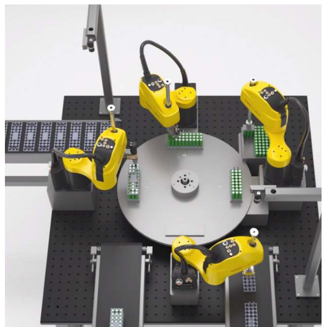
SR-3iA SCARA Robots assembling battery packs
