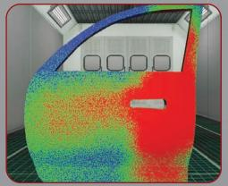
Coverage Map - View applied paint thickness vs. target mil build while the student paints.
