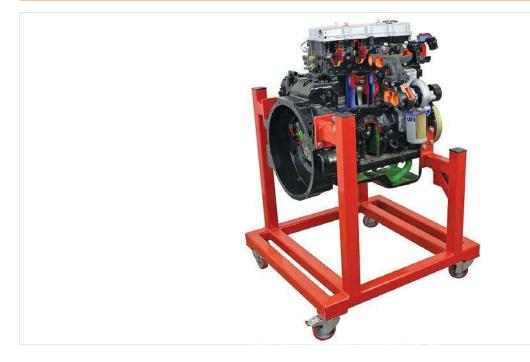
This trainer provides the instructor with a fully sectioned 4cylinder truck diesel engine for group or whole-class demonstration.
